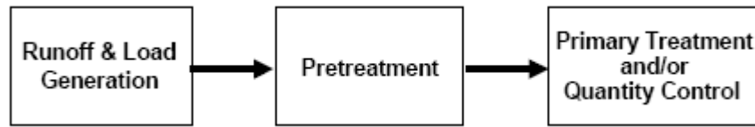
FIGURE 4-34 Generalized Stormwater Treatment Train
