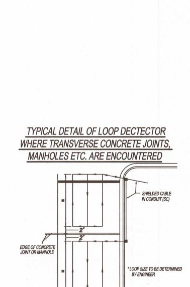
NO LOOPS ARE TO BE INSTALLED THROUGH, OVER, OR UNDER TRANSVERSE CONCRETE JOINTS IN CONCRETE PAVEMENT, AND NO MANHOLES, INLETS, ETC. MAY BE LOCATED WITHIN A LOOP. IF ANY OF THE ABOVE ARE ENCOUNTERED THE LOCATION OF THE LOOP MAY BE VARIED SLIGHTLY AS DIRECTED BY THE ENGINEER. IF THE ABOVE ITEMS ARE UNAVOIDABLE, SMALLER LOOPS AS SHOWN TO THE RIGHT MAY BE USED. SMALLER
