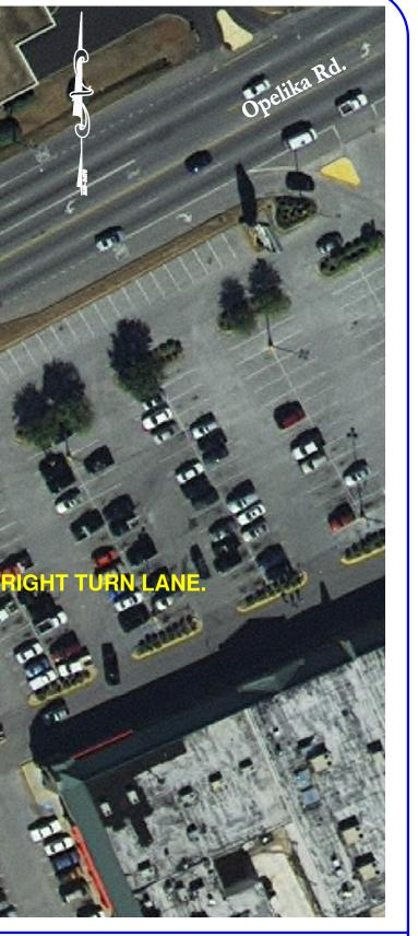
FIGURE 4 ALTERNATE ONE IMPROVEMENTS OPELIKA RD. AT E. UNIVERSITY DR. AUBURN TRAFFIC STUDY JUNE 2006 AUBURN, ALABAMA 1103.007 • Construct a right turn lane on southbound East University Drive to accommodate the right turn movement and provide access to the right turn lane during peak periods.
